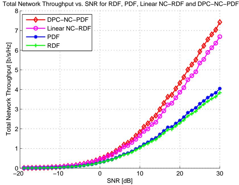
Figure 4: Total Network Throughputs of RDF, PDF, linear NC-RDF and DPC-NC-PDF
