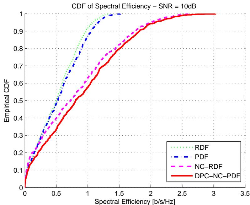
Figure 5: CDF of Spectral Efficiency - SNR = 10 dB
