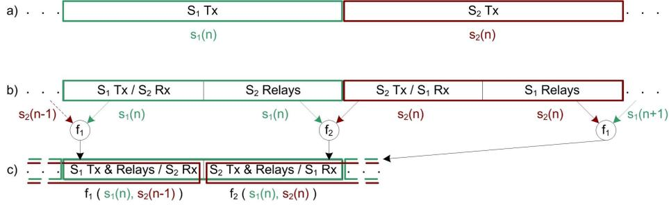
Figure 2: Time division channel allocations for (a) orthogonal direct transmissions, (b) usual orthogonal cooperative transmissions (c) proposed scheme : analog network coding cooperative transmissions
