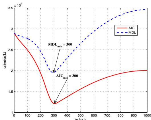
Fig. 4. The AIC and MDL of WiFi signal at 10 dB.
