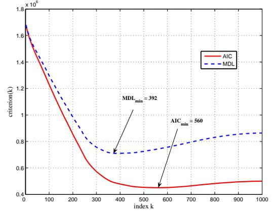
Fig. 2. The AIC and MDL of the UMTS Time Slot 1 (data).
