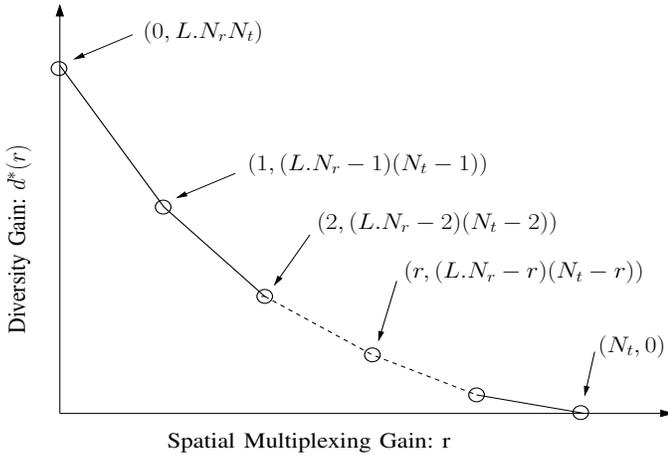
Fig. 3. Asymptotic diversity vs. multiplexing tradeoff for a frequency-selective channel (for the case  $N_t \leq N_r$ ).
