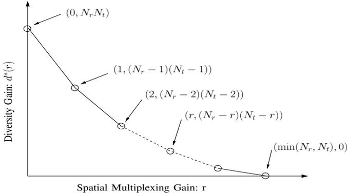
Fig. 2. Optimal Diversity vs. Multiplexing tradeoff (DMT) for freq.-flat MIMO ch.
