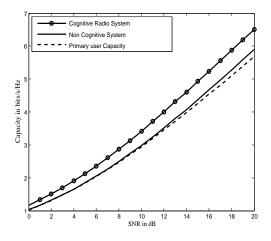
Fig. 2. Simulated capacities of the two configurations: with cognition and without cognition for N = 10.
