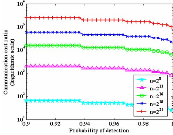
Figure 6. Communication cost ratio with varying number of segments.  $Data\_size = 30MB$ ,  $k/n=0.5$ ,  $hash\_size=128bits$ .
