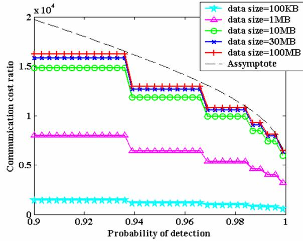
Figure 5. Communication cost ratio with varying data size.  $n=2^{16}$ ,  $k/n=0.5$ ,  $\text{hash\_size}=128\text{bits}$ .
