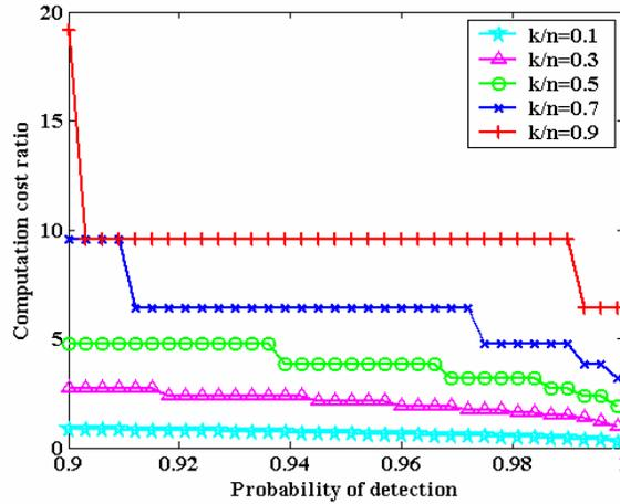
Figure 8. Computation cost ratio over probability of detection of misbehavior.  $Data\_size=65536$ bits,  $segment\_size=128$ bits, hash function: hmac-md5 [7]
