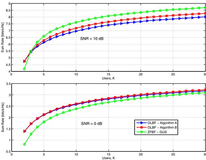
Fig. 3. Sum rate comparison of suboptimal beamforming approaches as a function of the number of users for  $M = 2$  transmit antennas, for a) average  $SNR = 0$  dB (below) and b) average  $SNR = 10$  dB (above).
