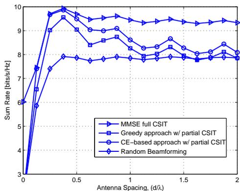
**Figure 2:** Sum rate as a function of antenna spacing for various user selection schemes with  $N_t = 2$ ,  $\sigma_\theta = 0.1\pi$  and  $K = 50$  users.
