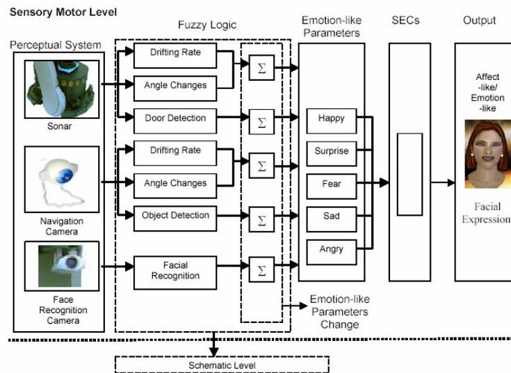
**Figure 5: Sensory Motor Level's sub-Architecture**
