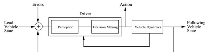
Figure 10: General Schema for Car Following Models
