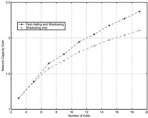
Fig. 3. Network capacity gain versus number of cells for different propagation scenarios. Gain increases with system size as optimization space increases. Greater channel variation increases performance gap between the two scheduling policies thereby increasing gain.
