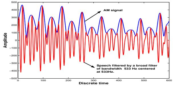
Fig. 3. The AM signal derived using broad-band filters
