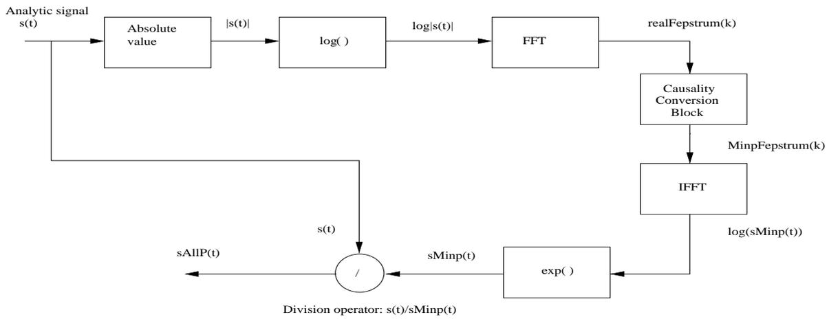
Fig. 1. Carrier signal decomposition via homomorphic filtering.
