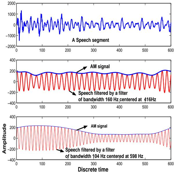
Fig. 2. The AM signal derived using narrow-band filters
