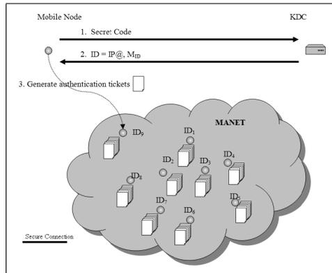
**Fig. 2.** Application of IB-MAC for naming and key management in open ad hoc networks.
