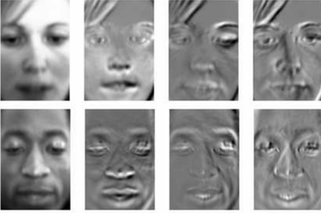
Fig. 7. Two different examples of individual user eigenfaces. In each row, the first 4 eigenfaces for the same user are shown, the first one including the mean face of the user.
