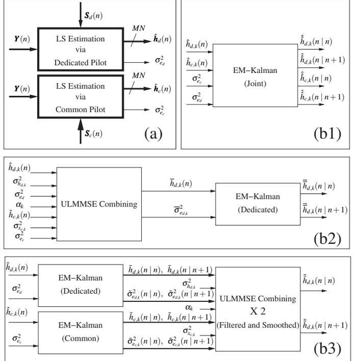
Figure 1: a: LS estimation (joint for all taps), {b1,b2,b3}: {optimal scheme, suboptimal scheme 1, suboptimal scheme 2} for each tap
