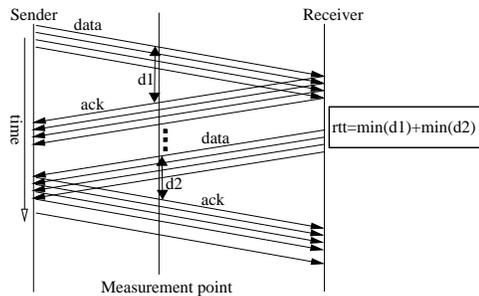
Figure 3: Round-trip time estimation using naive data-ack association.
