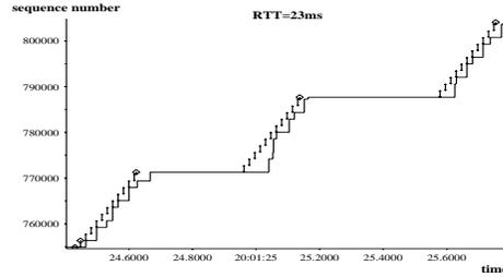
Figure 10: Rate limited BitTorrent connection.
