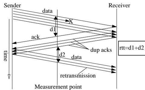
Figure 4: Round-trip time estimation using 3rd duplicate ack-retransmission association.
