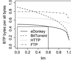
Figure 7: Fraction of all bytes in BTPs vs.  $lim$ .
