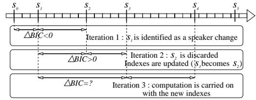
Figure 1: Principle of BIC final pass
