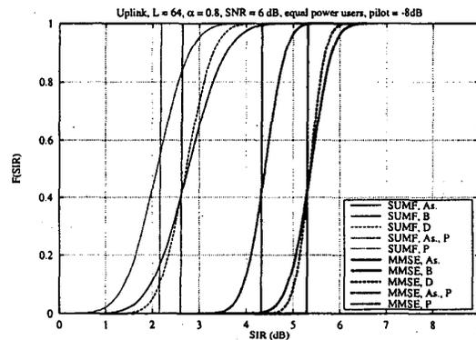
Figure 2: Cumulative distribution function of the SIR. Here  $L = 64$ ,  $\alpha = 0.8$ , SNR= 6 dB, and the pilot power to data power ratio equals -8 dB.
