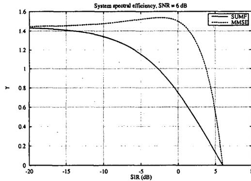
Figure 1: Asymptotic spectral efficiency  $\gamma$  of DS-CDMA vs. required SIR  $\beta_0$  (SNR = 6 dB).
