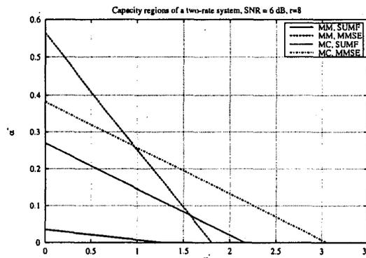
Figure 3: Asymptotic capacity regions for MM, MC (and approximately for VS) for random spreading sequences, SNR' = 6 dB, and rate ratio  $r = 8$ .
