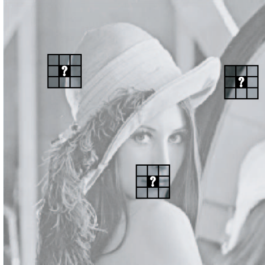
Figure 6.3: Error concealment techniques: when a block is detected as corrupted or missing, it is discarded and the algorithm tries to predict it using blocks in the vicinity.
