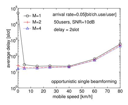
Figure 6: average delay vs. speed (B = 1 beamforming)
