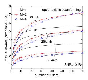
Figure 3: max sum-rate vs. number of users (beamforming with B=M)
