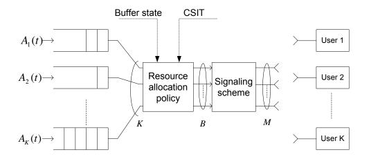
Figure 1: Block diagram of the SDMA/TDMA downlink
