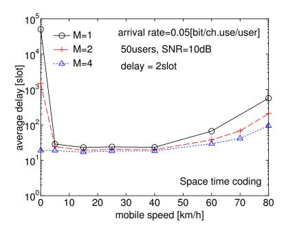
Figure 5: average delay vs. speed (STC)
