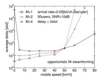
Figure 7: average delay vs. speed (B = M beamforming)
