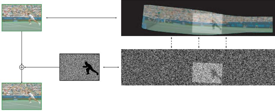
**Fig. 3.** Embedding procedure for camera motion coherent watermarking: The part of the watermark pattern which is associated with the current video frame is retrieved and registered back. Next, it is embedded in the background portion of the video frame.
