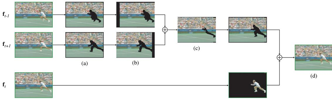
**Fig. 1.** BRA at the frame level: Once the video objects have been removed (a), neighbor frames are registered (b) and combined to estimate the background of the current frame (c). Next, the missing video objects are inserted back (d).
