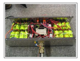
Fig. 11: Inside of the power supply box: from the 8 groups of 4 batteries the power supply passes through the red and violet cables, placed on purpose in those positions. The transformer, which provides power supply for the digital part (in acquisition state) and recharges the batteries (in recharging state), appears in the center of the box.
