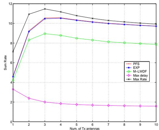
Figure 1. Sum Capacity versus the number of transmit antennas for a heterogeneous network with various QoS constraints.
