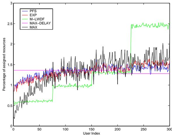
Figure 6. Frequency that each user with the corresponding SNR is chosen under different scheduling rules
