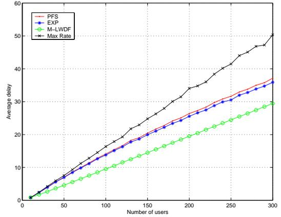
Figure 4. Average user delay (in ms) as a function of active users in the system. (Max delay performance is not shown for illustration reasons as its delay explodes and it is higher than all the others)
