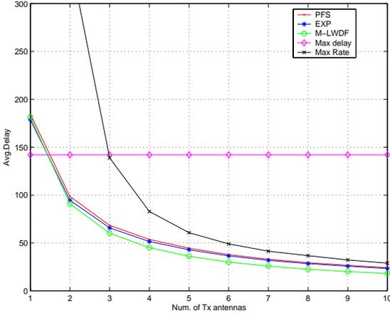
Figure 2. Average user delay (in ms) versus the number of antennas for a heterogeneous network with various QoS constraints
