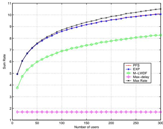
Figure 3. Sum Capacity as a function of the number of active users
