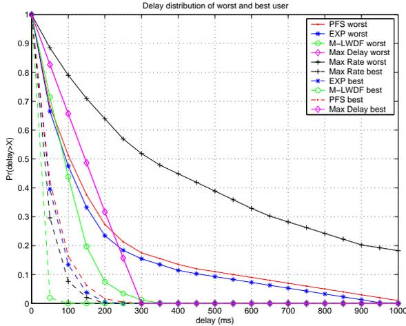
Figure 5. Delay distribution of the strongest and the weakest users of the heterogeneous network under different scheduling rules
