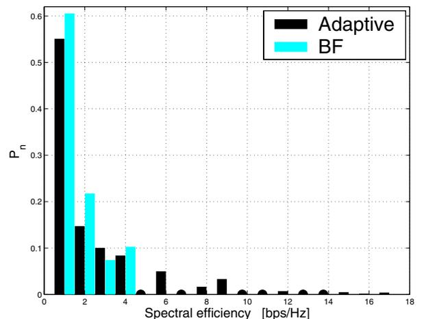
Fig. 2. Distribution of the downlink spectral efficiency for adaptive and fixed BF transmission techniques in channel Model 1.
