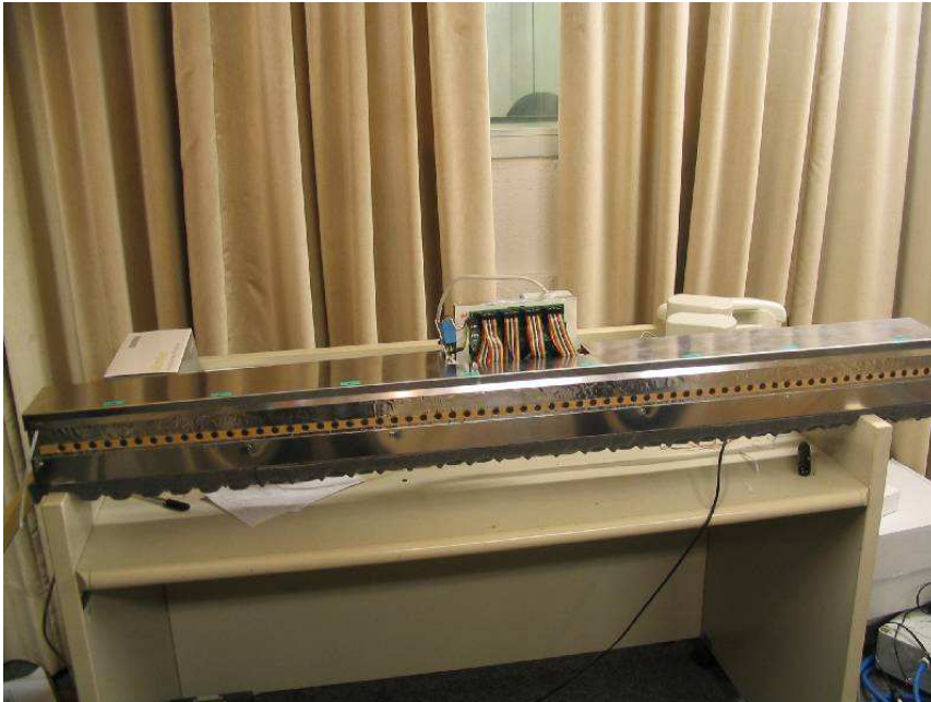
Figure B-4: the IRST-MarkIII after the intervention: an additional Faraday cage was added to isolate the last 50Hz noise residual.
