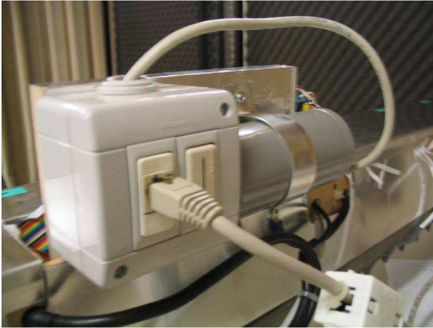
Figure B-7: The motherboard from behind: an Ethernet socket has been added for practical purposes only. The big 15 mF condenser is also visible.
