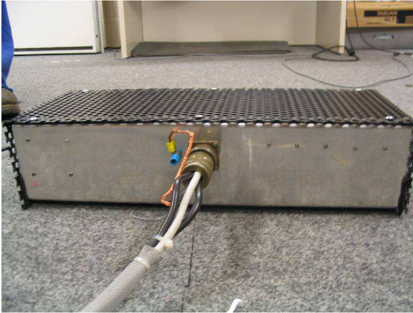
Figure B-9: Back of the power supply box: the ground is connected separately. The box is surrounded by a metal cage.
