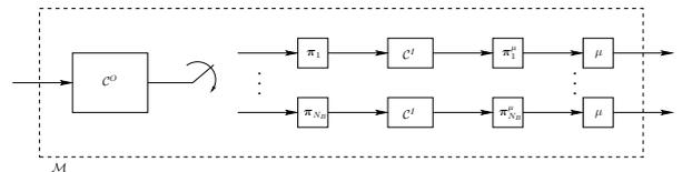
Fig. 2: Code structure for BCCs.
