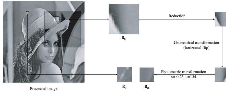
**Figure 5.** Block Replacement Attack (BRA): Each signal block is replaced by another perceptually similar one, e.g. modulo a geometrical and photometric transformation taken at another location.
