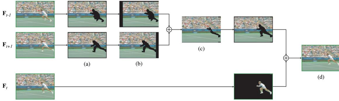
**Figure 4.** Temporal Frame Averaging after Registration (TFAR): Once the video objects have been removed (a), neighbor frames are registered (b) and combined to estimate the background of the current frame (c). Next, the missing video objects are inserted back (d).
