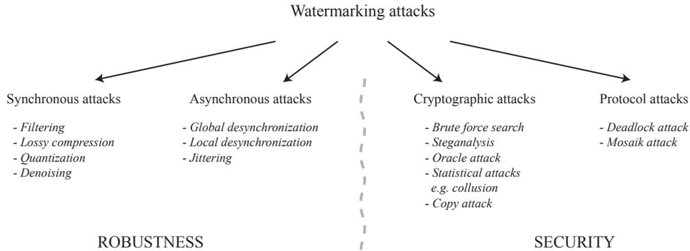
**Figure 1.** Watermarking attacks breakdown depending on whether they address robustness or security issues.
