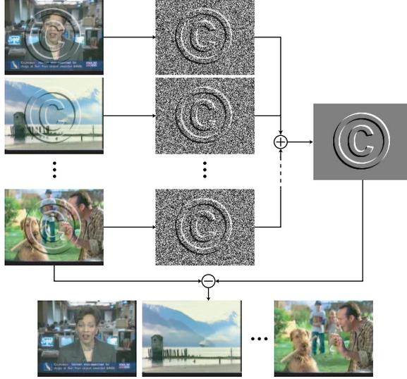
**Figure 3.** Watermark Estimation Remodulation (WER): Several watermark estimations obtained from different video frames are combined to refine the estimation and enable watermark removal.
