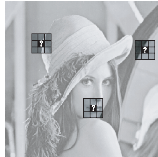
Figure 2: Error concealment techniques: when a block is detected as corrupted or missing, it is discarded and the algorithm tries to predict it using blocks in the vicinity.
