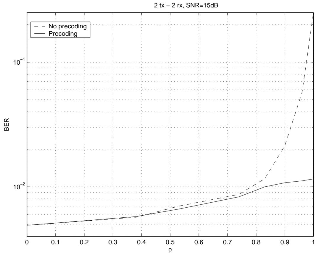
Fig. 7. 2 by 2 case. Improvement due to the proposed precoder with the ML receiver as function of correlation.
