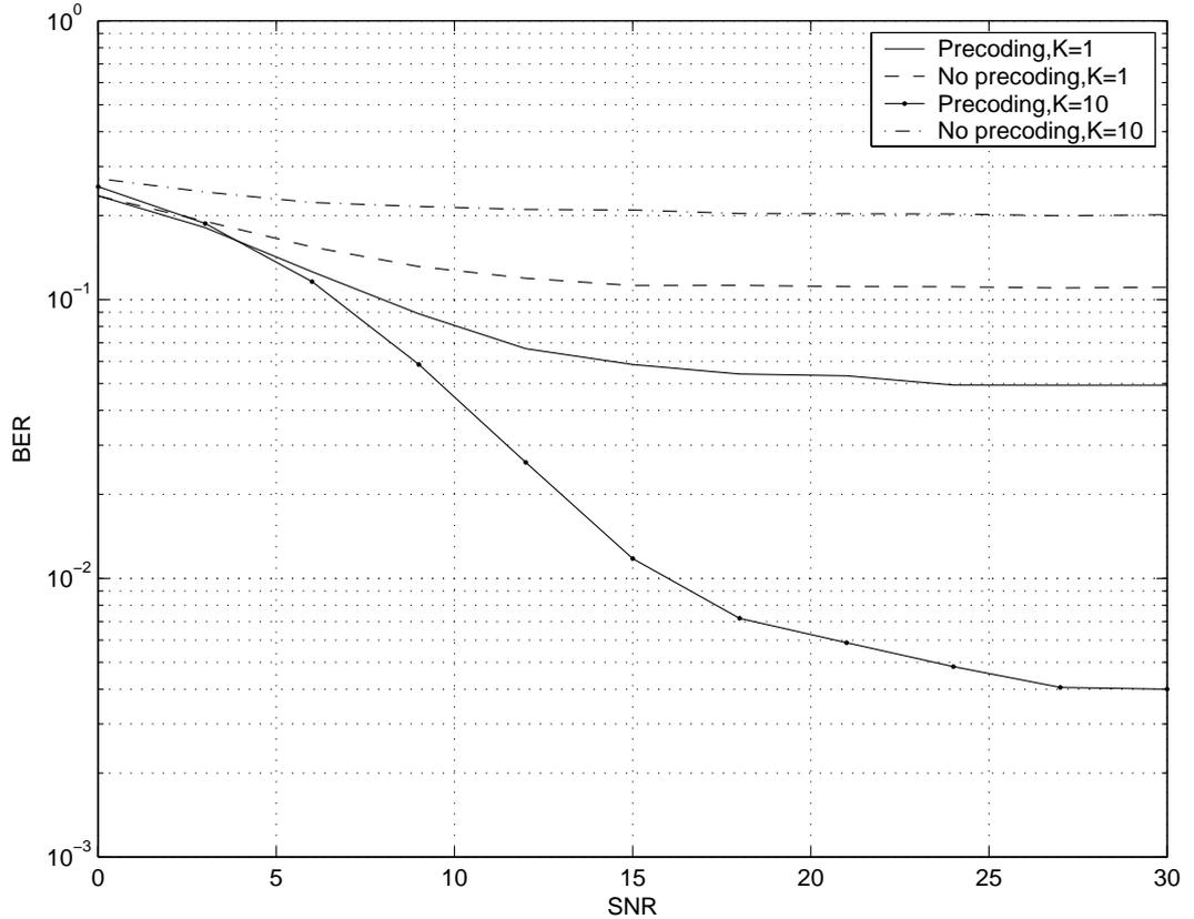
Fig. 3.  $K = 1, K = 10$ , MRC with/without precoding
