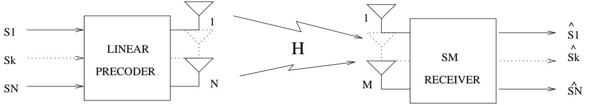
Fig. 1. Spatial multiplexing with precoding
