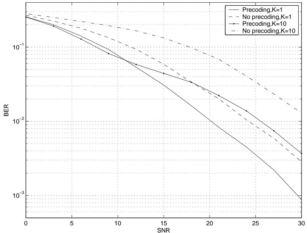
Fig. 5.  $K = 1$  and  $K = 10$ ,  $\rho = 0.8$ , MMSE SIC with/without precoding
