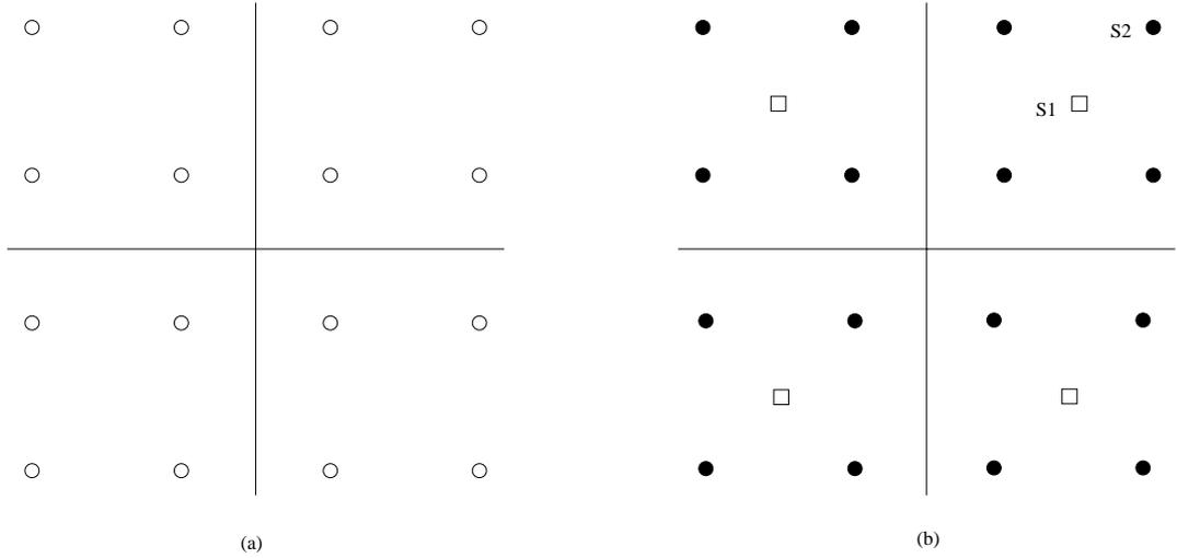
Fig. 2. (b): Illustration of two superimposed 4-QAM signals  $s_1$  and  $s_2$ . The latter is scaled down in power by  $1/4$ . (a): Resulting equivalent 16QAM constellation.
