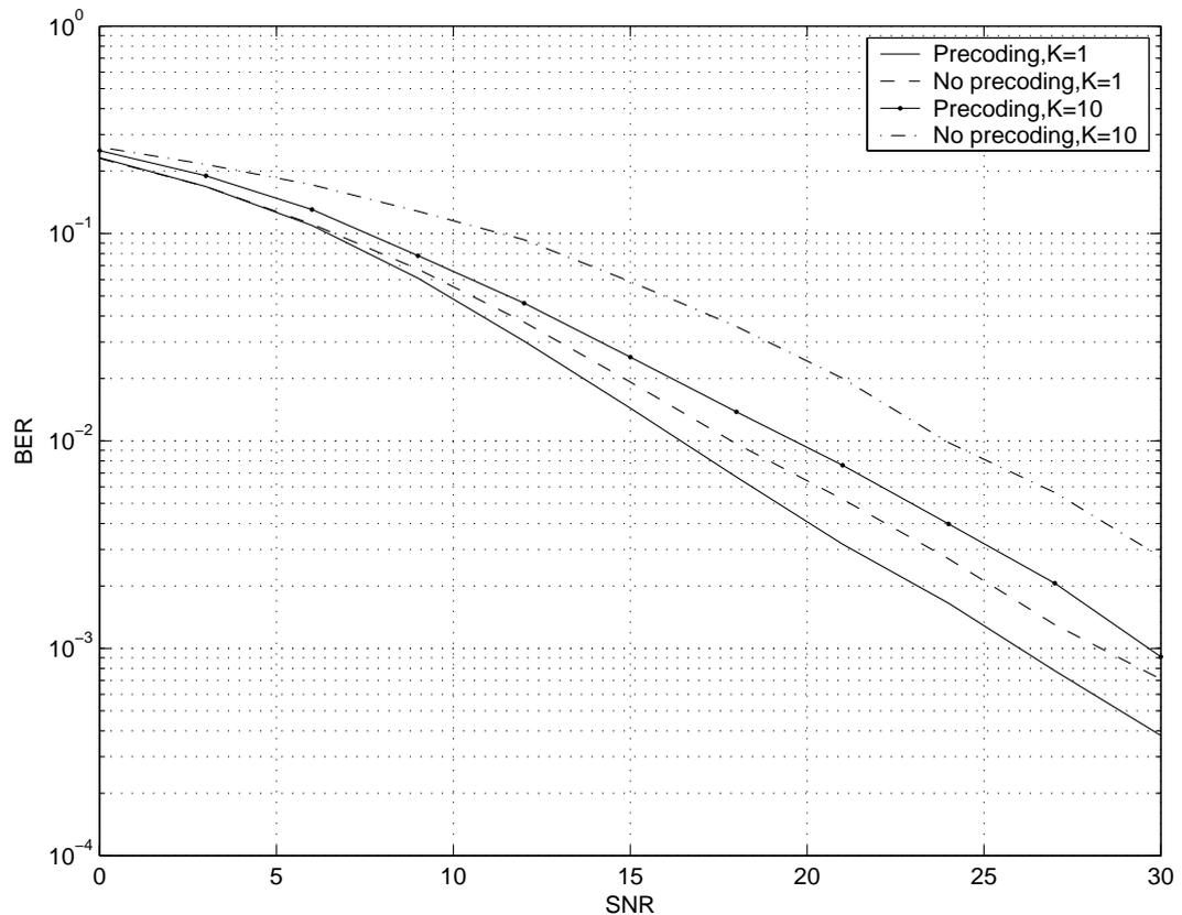
Fig. 4.  $K = 1$  and  $K = 10$ , MMSE SIC with/without precoding
