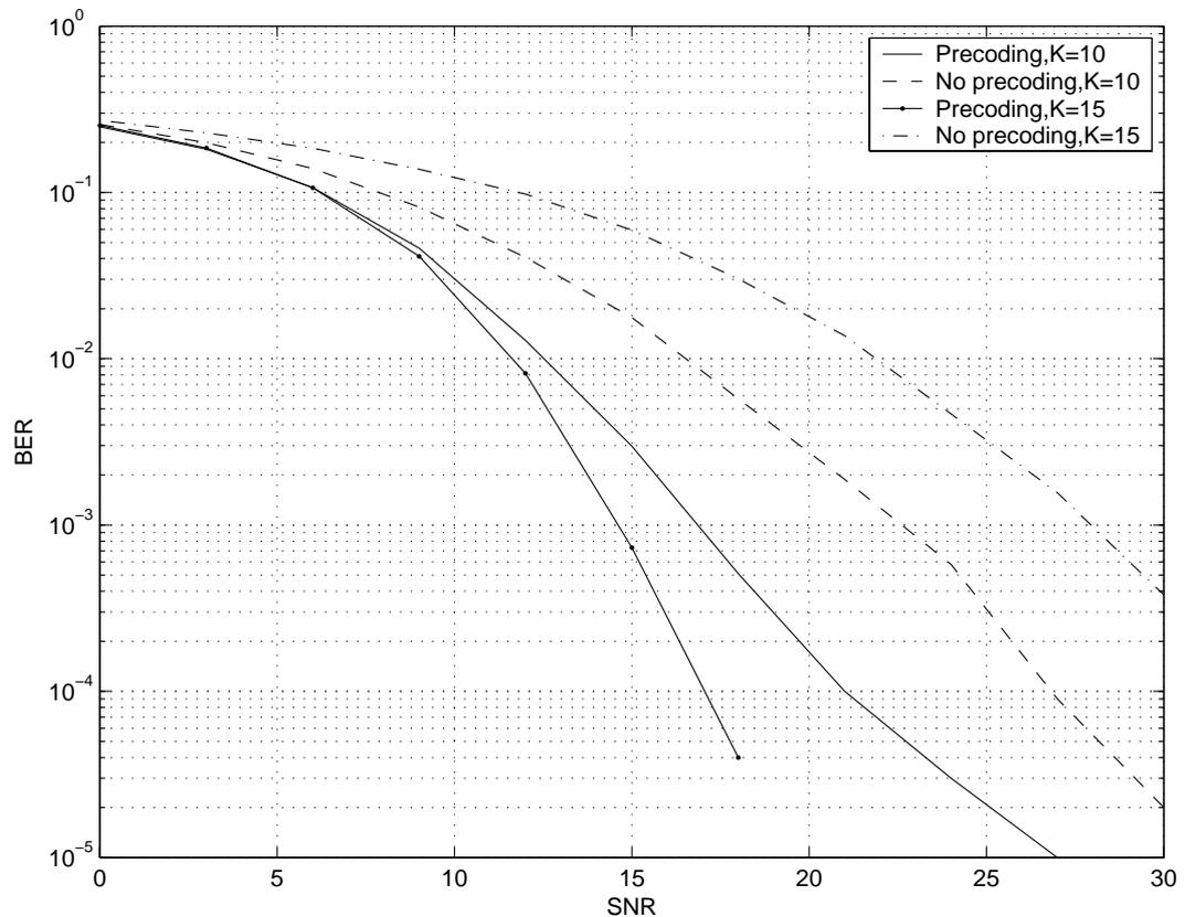
Fig. 6.  $K = 10$  and  $K = 15$ , ML with/without precoding
