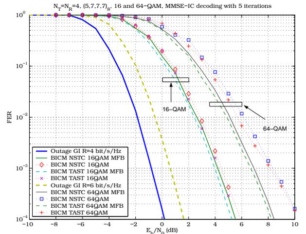
Figure 6: FER for  $N_T = 4$ ,  $N_R = 4$  with  $(5, 7, 7, 7)_8$  convolutional code, 16-QAM and 64-QAM with Gray mapping, with MMSE-IC decoding.
