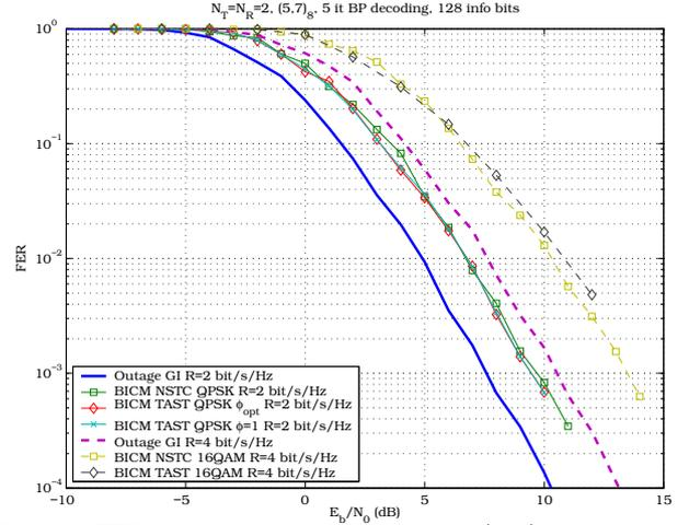
Figure 4: FER for  $N_T = 2$  and  $N_R = 2$  with  $(5, 7)_8$  convolutional code, QPSK and 16-QAM with Gray mapping.
