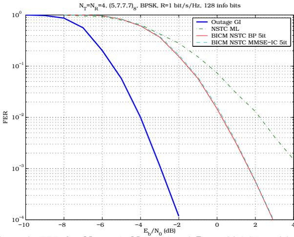
Figure 3: FER for  $N_T = 4$ ,  $N_R = 4$  and  $R = 1$  bit/s/Hz, with the  $(5, 7, 7, 7)_8$  convolutional code and BPSK modulation.
