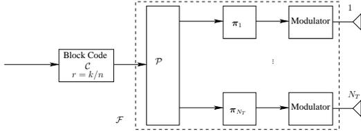
Figure 1: Transmission scheme of BICM NSTC.
