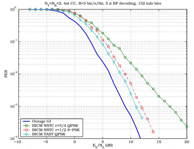
Figure 5: FER for  $N_T = 2$ ,  $N_R = 2$  and  $R = 3$  bit/s/Hz, with 4 states convolutional codes, QPSK and 8-PSK with Gray mapping.
