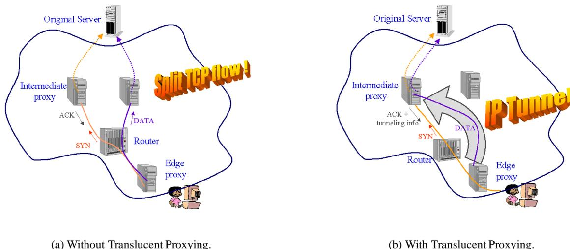
Figure 2: Translucent Proxying solves the Split Flow problem using IP Tunneling.
