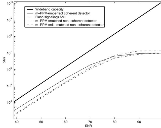
FIGURE 3. Achievable rates of energy detection based receivers+”flat” eigenvalues distribution:  $T_d=50$  ns,  $W=1$ GHz
