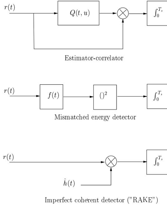
FIGURE 2. Receiver Structures
