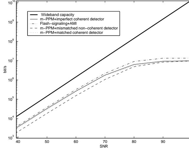
FIGURE 4. Achievable rates of energy detection based receivers+non-flat eigenvalues distribution:  $T_d=50$  ns,  $W=1$ GHz
