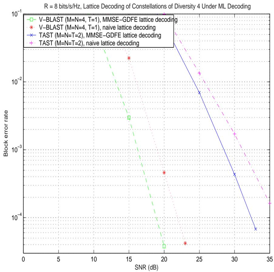
Figure 2: MMSE-GDFE lattice decoding versus naive lattice decoding.
