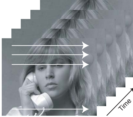
Fig. 8. Line scan of a video stream
