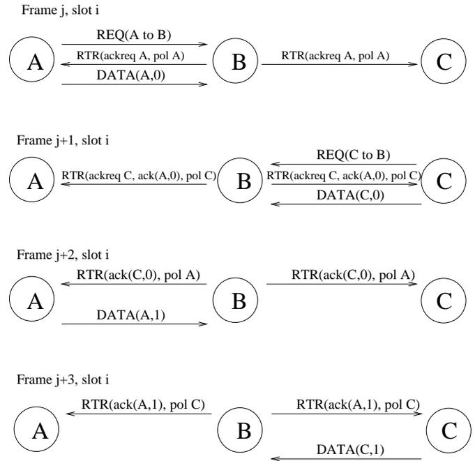
Fig. 2. Example of two parallel connections on a slot with CROMA
