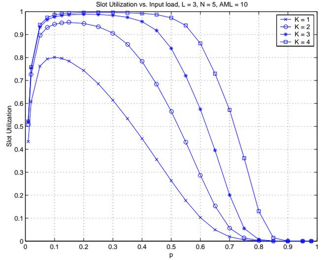
Fig. 7. Slot utilization vs. input load, influence of  $K$ ,  $L = 3$ ,  $N = 5$ ,  $AML = 10$
