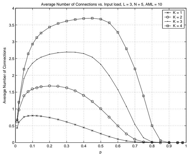
Fig. 8. Average number of connections vs. input load, influence of  $K$ ,  $L = 3$ ,  $N = 5$ ,  $AML = 10$
