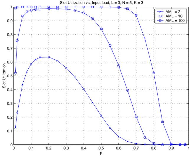
Fig. 6. Slot utilization vs. input load,  $L = 3$ ,  $N = 5$ ,  $K = 3$
