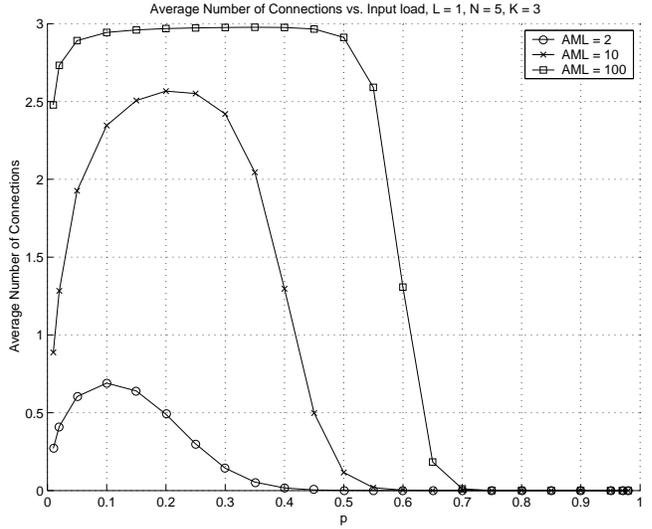
Fig. 5. Average Number of Connections vs. offered load,  $L = 1, N = 5, K = 3$
