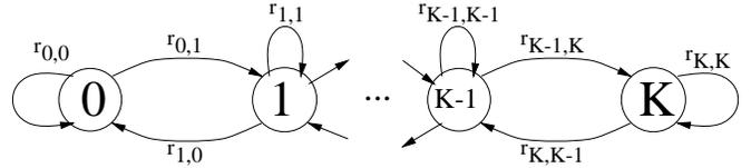
Fig. 3. Discrete time Markov chain representing the state of the slot, for  $N \geq K$ .
