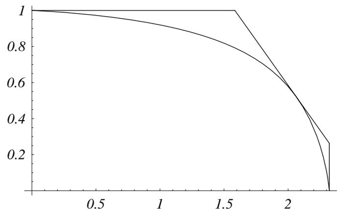
Fig. 1. Multiaccess channel capacity region and TDMA achievable region with with  $\text{SNR}_1 = 4$  and  $\text{SNR}_2 = 1$ .
