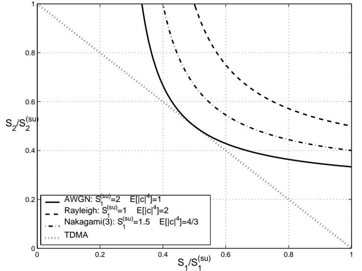
Fig. 6. Normalized slope region for the fading channel with  $\theta = 1$  and different fading statistics.
