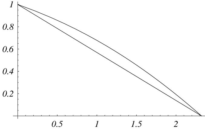
Fig. 3. Capacity region and TDMA-achievable rate region of broadcast channel with  $\text{SNR}_1 = 4$  and  $\text{SNR}_2 = 1$ .
