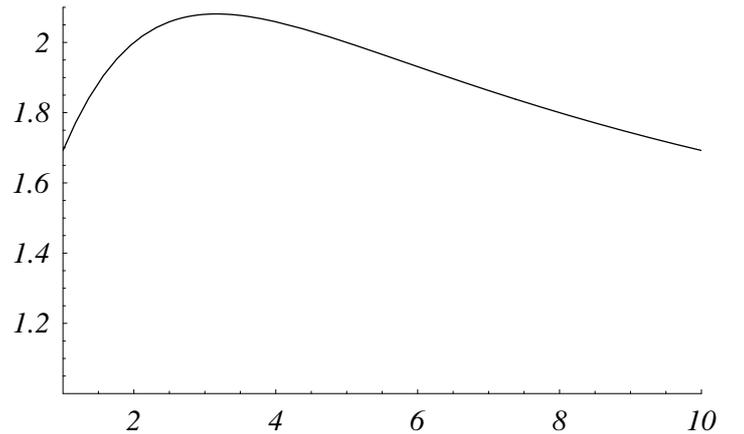
Fig. 7. Bandwidth factor penalty incurred by TDMA as a function of  $R_1/R_2 = \theta$  for  $|c_1|^2 = 10|c_2|^2$
