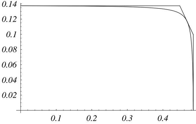
Fig. 2. Multiaccess channel capacity region and TDMA achievable region with with  $\text{SNR}_1 = 0.4$  and  $\text{SNR}_2 = 0.1$ .
