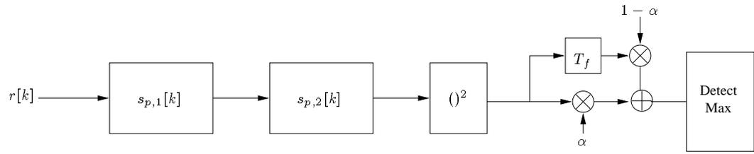
Figure 11: Primary Synchronization Processing
