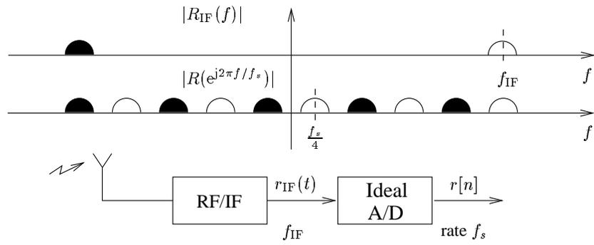
Figure 9: Receiver front-end
