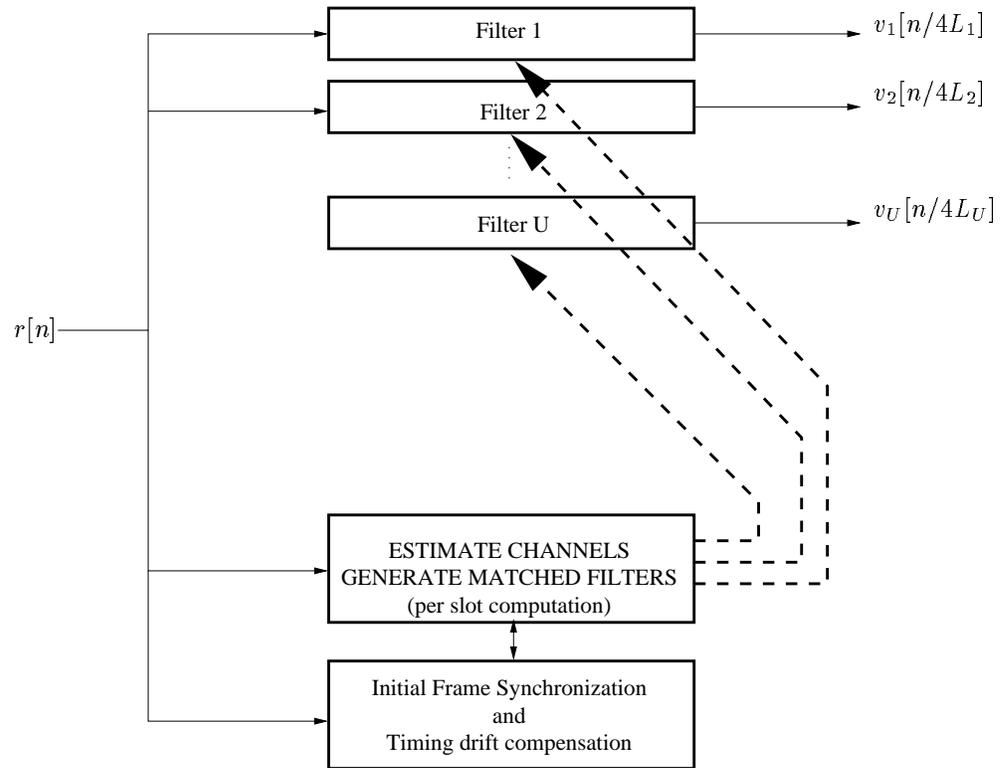
Figure 10: Basic RX structure
