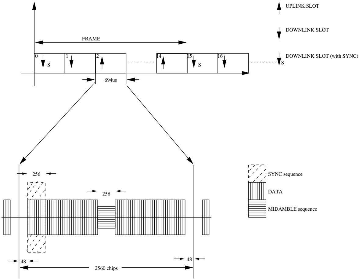
Figure 5: Slot structure
