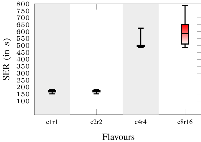
Fig. 10: SER for the URLLC service versus MME flavour. The box plot includes the 10 th , 25 th , median, 75 th , and 90 th percentiles of these times
