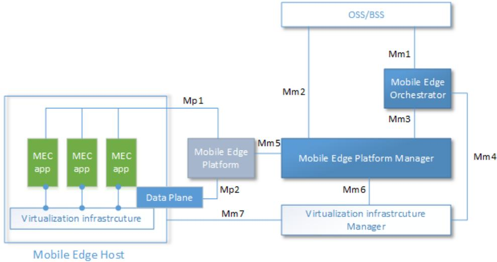
Fig. 1. High-level representation of the MEC architecture (based on [5]).
