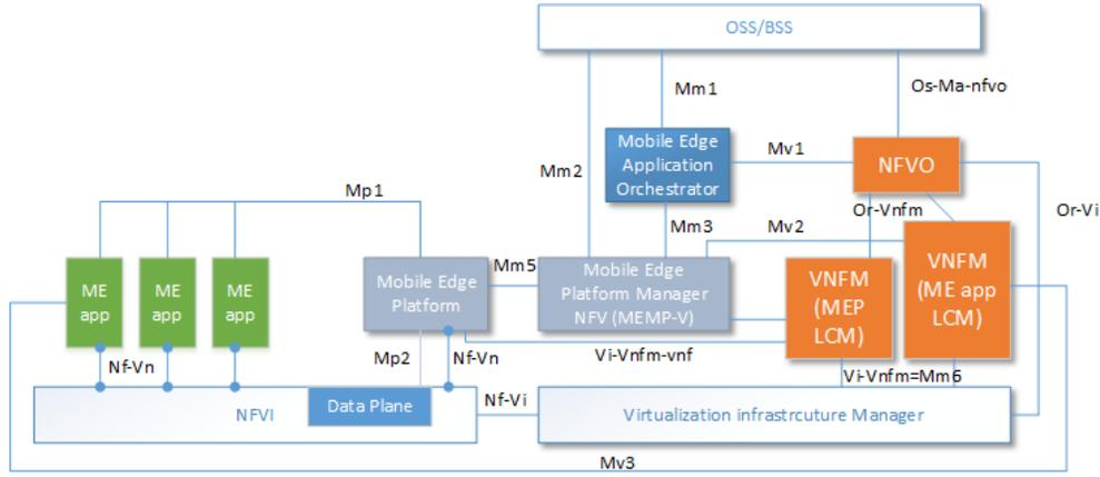
Fig. 2. Updated version of the MEC architecture featuring MEC in NFV (based on [4] and [5]).
