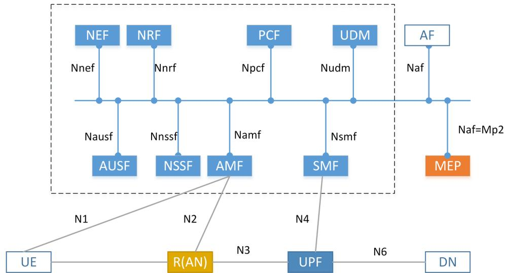
Fig. 3. 5G Core Network service-oriented architecture.
