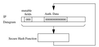
Fig. 5. Computation of the Authentication Data Field for AH
