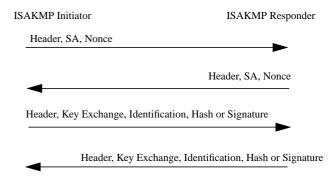
Fig. 16. Message flow for the base ISAKMP exchange
