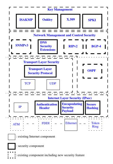
Fig. 1. Crtyptographic security components of the Internet infrastructure
