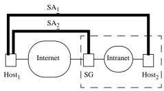
Fig. 12. Remote access with IPsec
