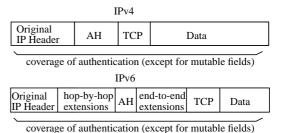
Fig. 3. Transport mode AH placement in the IP datagram
