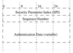
Fig. 2. Main fields of the IP Authentication Header
