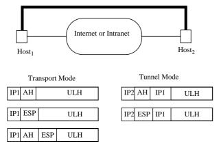
: one or more SA's applied to the same traffic stream IP1: original IP header IP2: encapsulating IP header ULH: Upper Layer Header
