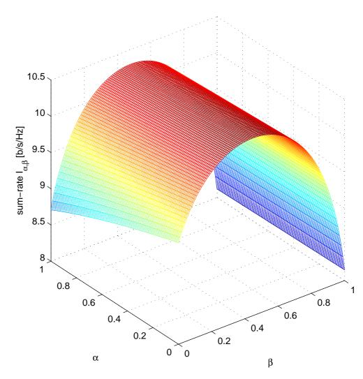
Figure 4: The sum-rate, in centralized case and linear network, when the mobile 2 is located at (0.1,0) and SNR equal to 10 dB. The centralized algorithm gives (0,0.446) as optimal power allocation indicating that only mobile 2 will cooperate.
