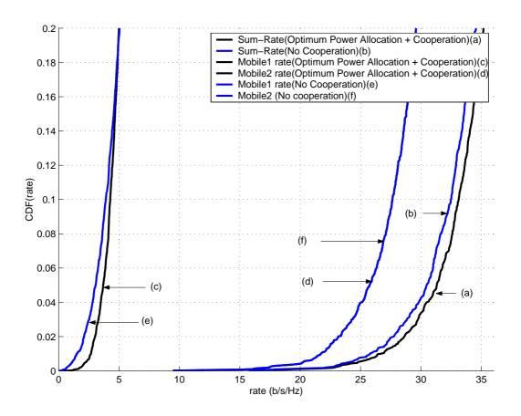
Figure 10: Outage capacity in centralized case and asymmetric network with user 2 located at (0.9,0), i.e, close to the destination; both the sum-rate and user 1's rate benefit from the cooperation, while user 2 almost never uses user 1 as a relay.
