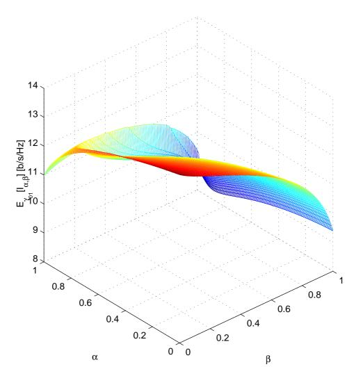
Figure 6: Expected sum-rate seen by mobile 2 (distributed processing) when it is located at (0.1,0) in linear network and SNR equal to 10 dB. The relations in (11) give (0,0) as optimal power allocation for mobile 2, therefore it should not cooperate.
