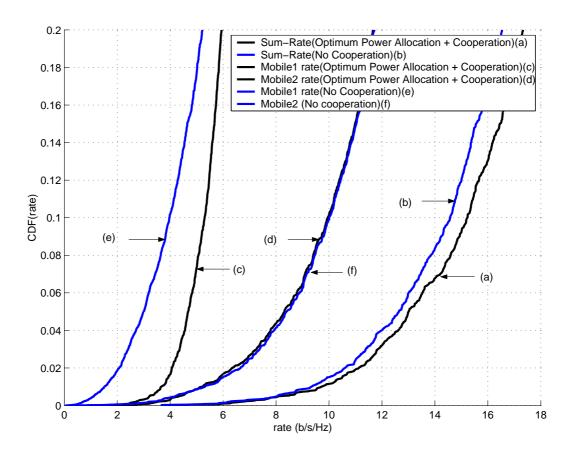
Figure 9: Outage capacity in centralized case and asymmetric network, with user 2 located at (0.5,0), i.e, halfway between user 1 and destination; Only user 1 benefits from cooperation, however the sum rate is also improved.
