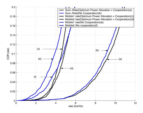
Figure 8: Outage capacity in centralized case and asymmetric network, with user 2 located at (0.1,0), i.e, close to the user 1; Both users as well as the sum rate benefit from cooperation, especially mobile 1.
