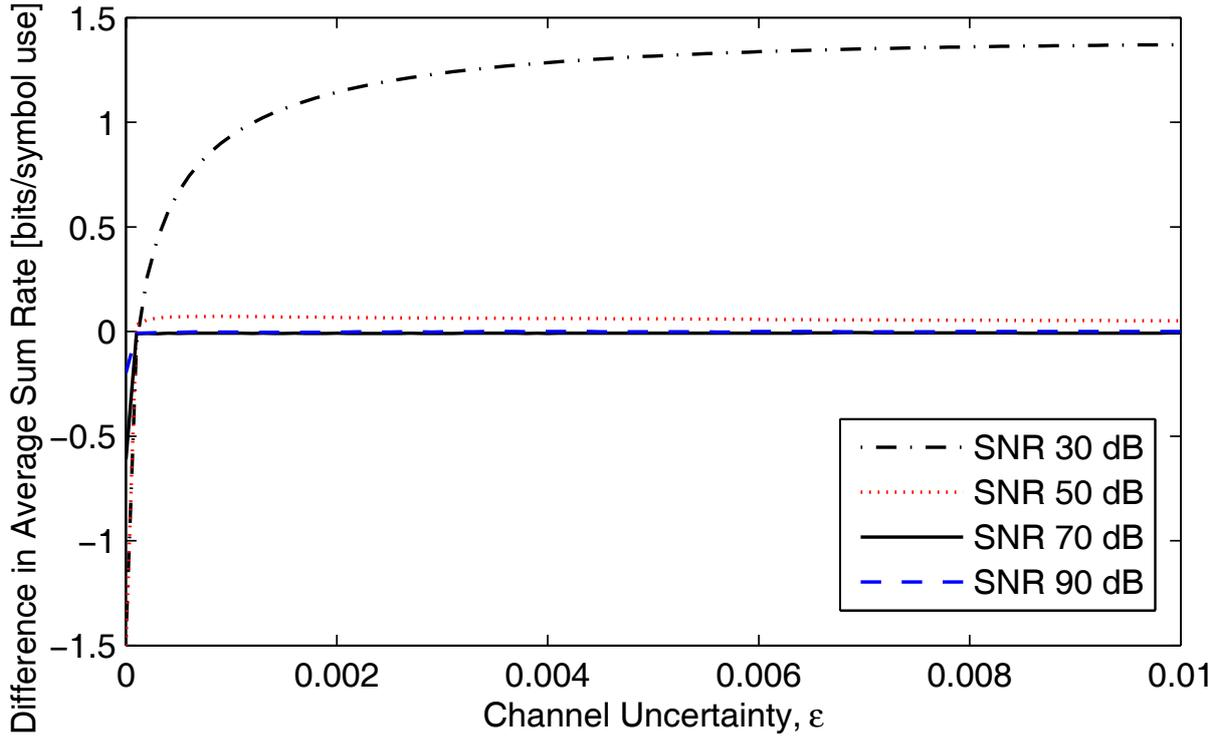
Fig. 5. Difference in average sum rate between LVSINR and ZF for small perturbations in the CSI used for precoding design. Same scenario as in Figure 4(a) with  $K_t = K_r = N_t = 4$ . Positive value means higher performance with LVSINR.
