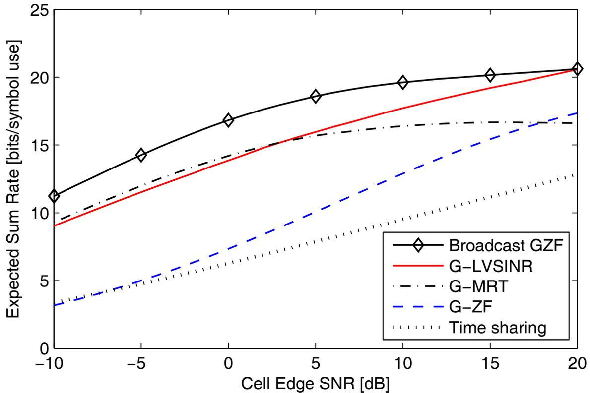
Fig. 6. Expected sum rate (over terminal locations and channel statistics) in a system with local statistical CSI,  $K_t = K_r = 4$ ,  $N_t = 6$ , and an angular spread of 10 degrees (as seen from each base station). The scenario considers uniformly distributed terminals within a square with base stations in each corner.
