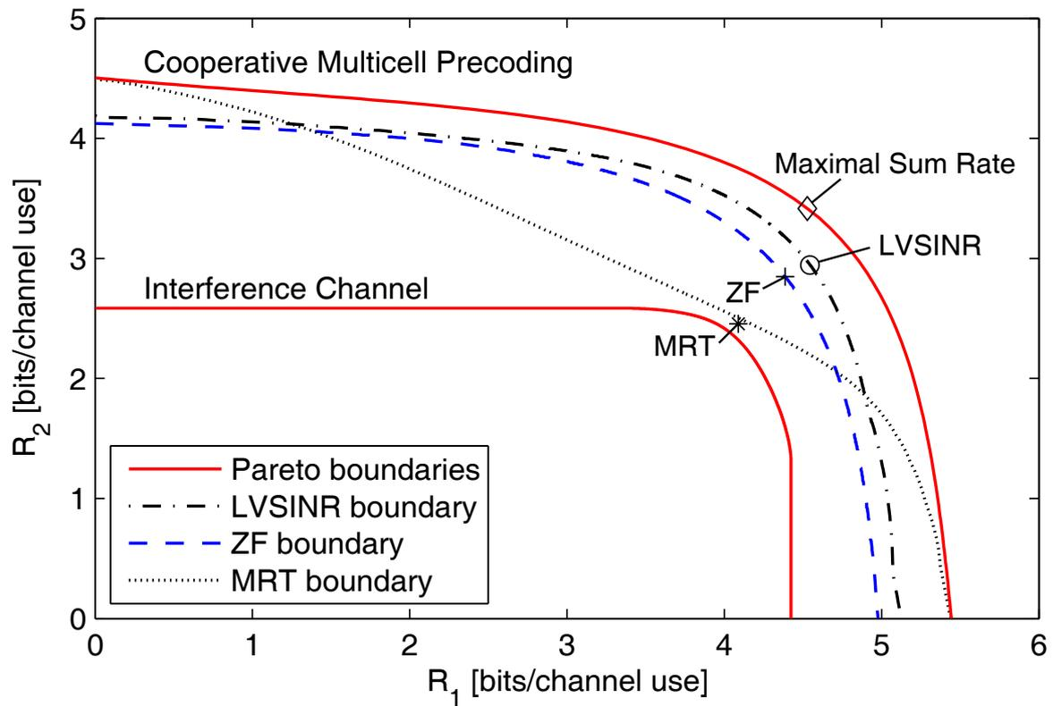
Fig. 2. Achievable rate regions with different beamforming and power allocation for  $K_t = K_r = 2$ ,  $N_t = 3$ , and a random realization with  $\mathbf{Q}_{11} = \mathbf{Q}_{22} = \mathbf{I}$ ,  $\mathbf{Q}_{12} = \mathbf{Q}_{21} = 0.5\mathbf{I}$ , and SNR 5 dB. The sum rate point and the points achieved by MRT, ZF, and LVSINR with the power allocation in Strategy 2 are shown for comparison.
