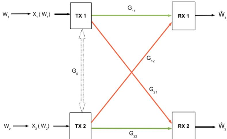
Figure: The interference channel with possible transmitter cooperation.
