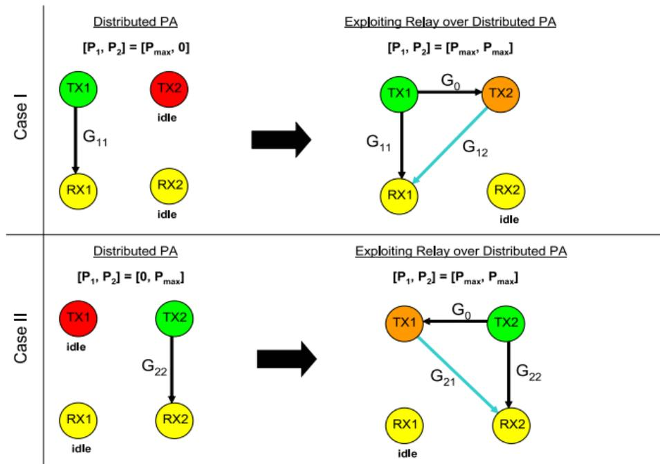
Figure: Two cases for which relaying mechanism is used after DPA.
