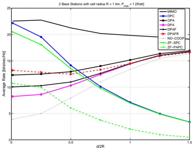
Figure: Average sum-of-rates vs.  $d/2R$  for Circular cell layout.
