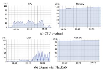
Fig. 8: PyVMMonitor profiling reports for JOX footprint
