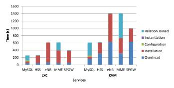
Fig. 10: Deployment time of VNF chains
