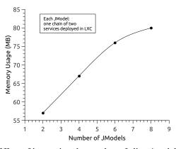
Fig. 9: Effect of increasing the number of slices/models on the memory usage. Every model is a chain of two services (either mysql-OAI HSS, or mysql-apache2) deployed in LXC.
