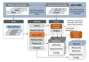
Fig. 3: JOX main components and properties
