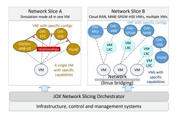
Fig. 1: JOX support for two network slices. In *slice A* the OAI eNodeB and EPC are deployed in a single VM. In *slice B* a cloud-RAN chain using disaggregated RAN is deployed over different VMs.
