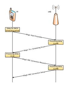
Fig. 2. Random Access CHannel (RACH) procedure
