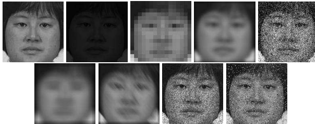
Figure 2: Obscured face images with filters. From left to right on the top: clean faces, blackener, pixelization, gaussian blur, gaussian noise; on the bottom: average blur, motion blur, speckle noise, salt and pepper noise.
