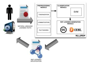
Fig. 1. The architecture of NLL2RDF.
