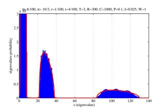
Fig. 1. Asymptotic eigenvalue distribution of the matrix  $\mathbf{Y}\mathbf{Y}^{\dagger}/R$  in solid red line for  $\alpha = \frac{1}{100}$ ,  $\kappa = \frac{10}{3}$ , P = -10 dB,  $I_k = \frac{P}{4} \forall k$ , W = 0 dB. The asymptotic eigenvalue distribution is compared to the empirical eigenvalue distribution for T = 3, R = 300, and C = 1000 given by the histogram in blue.
