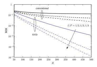
Fig. 5. BER vs. number of receive antennas with T = 3, C = 1000, L = 2, and P/W = 0.1 (SNR is -10 dB).
