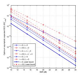
Fig. 3. The impact of spatial correlation on optimum asymptotic expected EED.  $N_t = 4$ ,  $N_r = 2$ ,  $\eta = 0.2$ , and  $P_s = 1$ .
