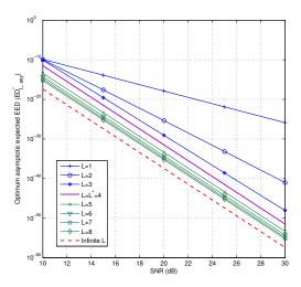
Fig. 2. The impact of frequency diversity on optimum asymptotic expected EED. The channel is uncorrelated,  $N_t = 4$ ,  $N_r = 2$ ,  $\eta = 0.2$ , and  $P_s = 1$ .
