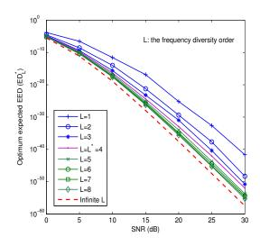
Fig. 1. The impact of frequency diversity on optimum expected EED. The channel is uncorrelated,  $N_t=4,\,N_r=2,\,\eta=0.2,$  and  $P_s=1$
