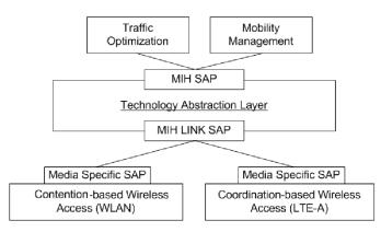
Fig. 1. MEDIEVAL Wireless Access Architecture and Cross-layer Design
