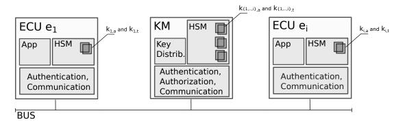
Fig. 1. Simplified deployment architecture. One ECU acts as Key Master node (KM). Symmetric keys are shared with every other ECU ( $e_1$ ,  $e_i$  shown). All keys reside in the corresponding HSM. System wide policies are evaluated at the key master (Authorization).
