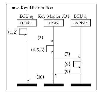
Fig. 2. Key Distribution via Key Master. Steps (6-9) are executed for all i ECUs in the receiver group. The numbers correspond to the steps defined in III-A.
